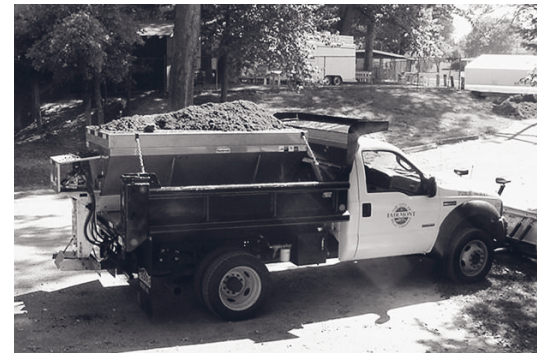
Abrasives have been pre-loaded on this truck. Photo by Emily Walters from WV LTAP's 2005 Snow and Ice Control Workshop.
