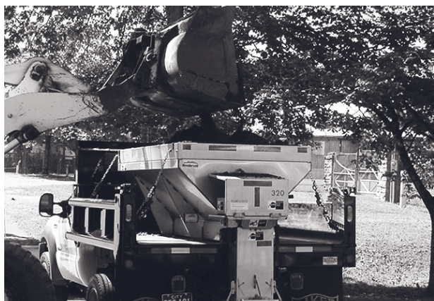
Abrasives are being loaded into a truck. Photo by Emily Walters from WV LTAP's 2005 Snow and Ice Control Workshop.
