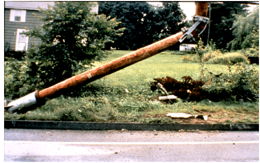
Post-Crash View of Breakaway Pole (Massachusetts)
